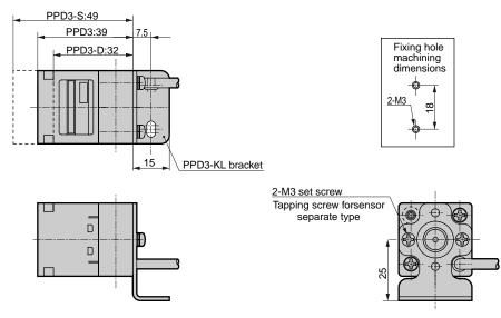
PPD3-KD (-D)-P70 assembly drawing Note: With this installation, use the CKD miniature joint FTL4-M3-P70 for the atmospheric pressure introduction port joint. (Only sensor integrated type)
