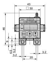
Fixing hole machining dimensions <u>2-M3</u>
