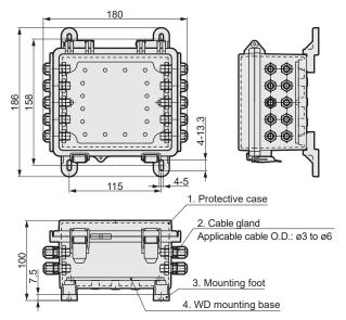
The outline drawing shows the state where the following parts (No. 2 to 4) are attached to the protective case. Please install each part by yourself.
