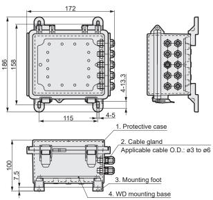
The outline drawing shows the state where the following parts (No. 2 to 4) are attached to the protective case. Please install each part by yourself.
