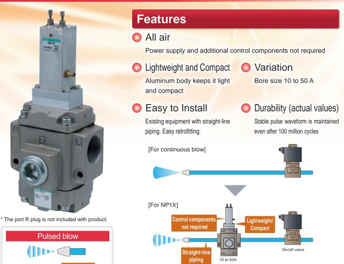
Can be converted to Pulse Blowing Circuit by simply adding this product to the continuous blowing piping.
