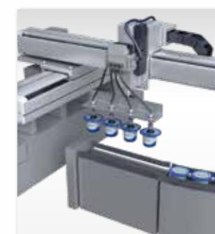
A vacuum ejector unit designed for high-speed operation.
