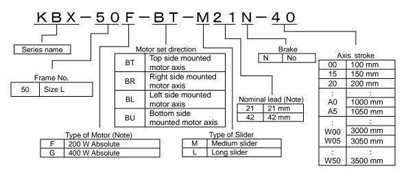
Note 1: Compatible only with the 21 mm-lead product in the case of a 200-watt motor. Compatible only with the 42 mm-lead product in the case of a 400-watt motor.
