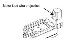
(16) Mount the motor on the motor block, and loosen four bearing clamping plate screws on the bottom of the motor block. Make sure that the bearing clamping plate rotates a little about the bearing. After that, uniformly retighten bearing clamping plate mounting screws having been loosened. Make sure that there is no misalignment between the motor mounting position and bearing clamping plate. (For the 21 mm-lead product, this work is not necessary).
