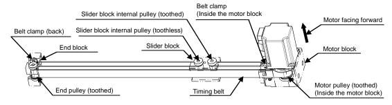
• Bottom side mounted motor axis
