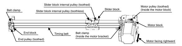
• Left side mounted motor axis (The end side belt clamp is located inside the end base.)
