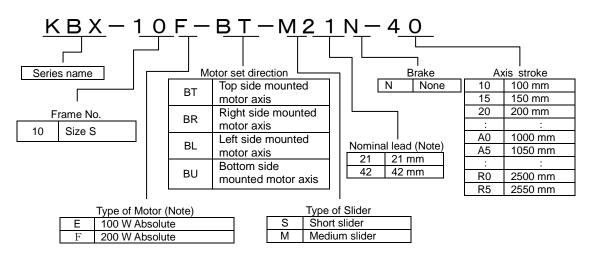
Note 1: Compatible only with the 21 mm-lead product in the case of a 100-watt motor
