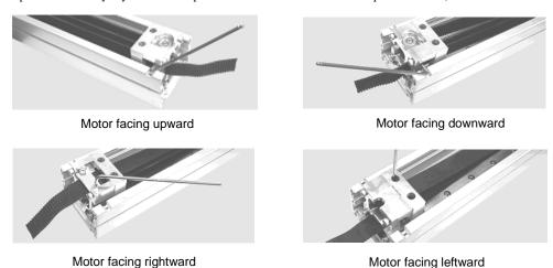
(3) Loose the bolt on the motor output shaft side of the coupling located inside, from the hole of the motor spacer. (For the 42 mm-lead product, this work is not necessary.)
