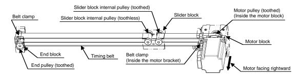
• Left side mounted motor axis (The end side belt clamp is located inside the end base.)
