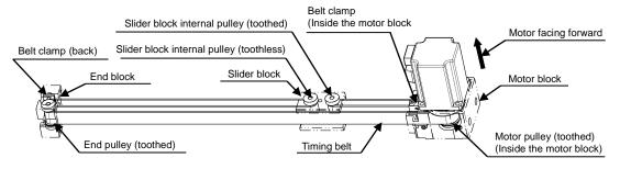
• Bottom side mounted motor axis
