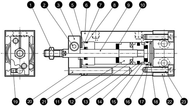
Note: Do not move the position of baffle plate (3) when using.
