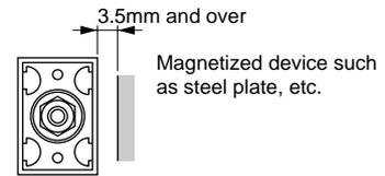
■ When installing cylinders adjacently, provide the following installation pitch to prevent switches from malfunctioning.
