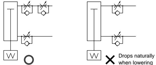
(Note 3) Connect the speed control valve in the parallel with the following circuit.
