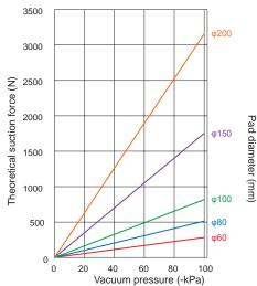
\*Depending on the pad shape, there are pads with no setting for the pad diameter indicated in the graph. Check the size with the pad size list in the table below.
