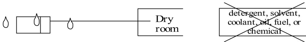
**CAUTION** : Do not apply pressurized air to the atmosphere pressure lead-in port. Doing so may cause the product to break or to be damaged, resulting in scattering of case parts.
