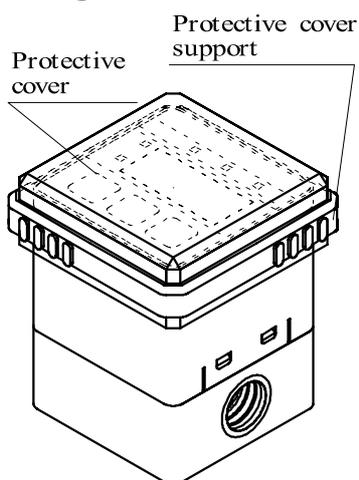
Pick and pull the projections on the both sides of the protective cover (approximately 2 mm) to mount or remove the cover.
