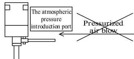
The atmospheric pressure introduction port of the models PPD3(-S)-\*\*\*\*\*-6B and 6T uses M3 screws. Therefore, use the following parts for these models. CKD Barb joint, DTS4-M3, FTL4-M3
