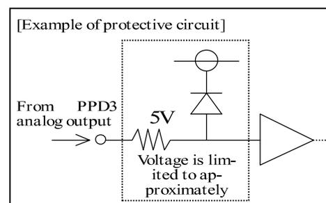
Note : Normally, the analog input system is constructed by power voltage of up to 15V. If an analog power voltage of 24V is applied to an electronics part, such as operational amplifier IC, a trouble called “latch up” may occur in the worst case, causing a large current to flow, resulting in burning of IC and power supply circuit.
