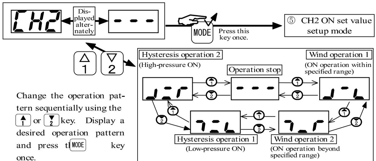
Change the operation pattern sequentially using the  $\uparrow$  or  $\downarrow$  key. Display a desired operation pattern and press the  $\text{MODE}$  key once.
