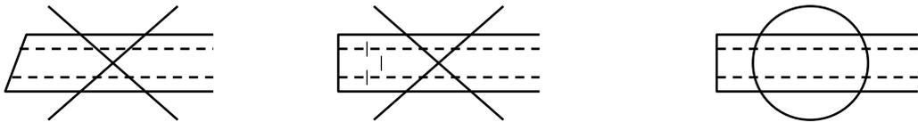
Cut the tube slantwise. Damage, contamination, and/or deformation Cut the tube straight.
