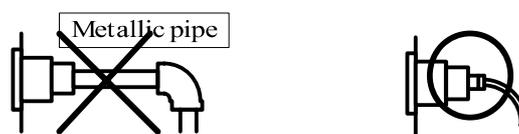
Accordingly, do not apply any tensile force, vibration, and/or impact to the tube after mounted. Do not connect a long tube, which may be suspended. Doing so may cause unexpected stress by vibration or impact. When using a long tube, secure it to the frame around the switch and connect it to the product after it is connected using the relay connection joint.
