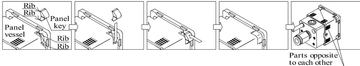
Four panel keys are put as they are connected to the runner. Cut the panel keys using diagonal cutters, and then attach them. Additionally, the runner is used as a handle and attach the panel key to the opening part. After that, cut the panel key or turn the runner part to twist and cut the panel key while pressing it.
