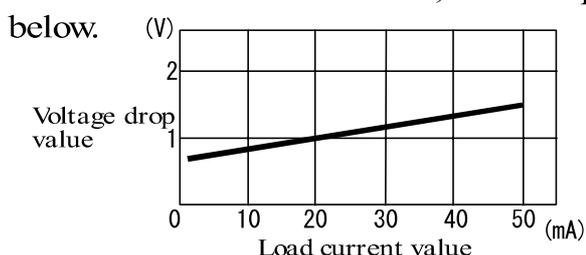
Note: As a protective circuit is added, the voltage drop may become approximately 1V higher than that of the conventional model. However, this may not affect the PLC input. For safe operation, always check the specifications for the input unit.
