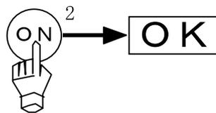
This product does not detect the pressure immediately after the power is turned ON. The control circuit is so designed that the signal is ignored for approximately 2 sec. after the power is turned ON.
