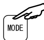
The setup operation is stopped and operation returns to the normal pressure display without recording of changed data.
