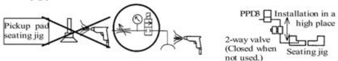
When flushing the piping to remove dust, supply the air, the pressure of which is regulated so that it does not exceed the proof pressure of the product or peripheral device.
