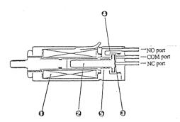
When the coil ①is deenergized, the plunger ② is returned to its original position due to the resiliency of the spring ⑤ to cause the valve seat ④ to be opened, and the valve seat ③ to be closed, thereby causing a fluid to flow to NO↔COM.
