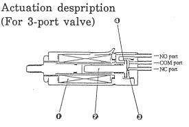
When the coil ①is energized, the plunger ② is attracted to cause the valve seat ③ to be opened, and the valve seat ④ to be closed, thereby causing a fluid to flow to NC↔COM.
