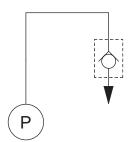
Prevents back flow during control of 2 kinds of fluids Prevents the back flow in circuits where fluids of different pressures and types merge.
