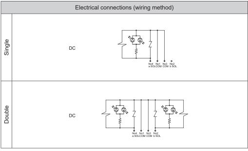
Note: Only available with a rated voltage of 24 VDC and with surge suppressor and indicator lamp.
