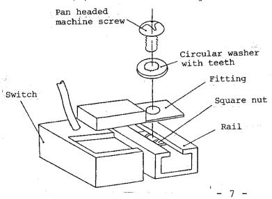
The criterion for the tightening torque of pan headed machine screw is 5 - 7 kgf-cm. Loosen slightly for shifting.
