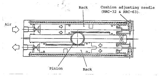
Selex Rotary is a rack pinion type rotary actuator. It conveys the reciprocating motion of the rack, corresponding to the straight cylinder piston, to the pinion, converts the motion into rotary motion to achieve oscillating motion of the output shaft.
