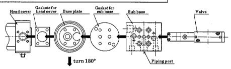
SCA2-V2 (Retracting type when energized · Single solenoid type)
