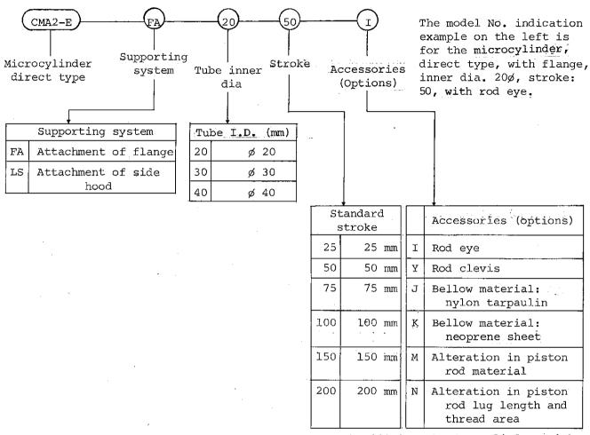
Stroke 200 is only for cylinders with tube inner diameters of 30% and 40%.
