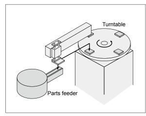
Two electrical components sorted by the parts feeder are simultaneously vacuum-suctioned and transported to the jig on the turntable for assembly.
