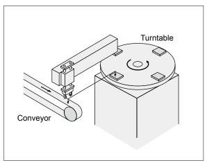
Vehicle components fed down the conveyor are transported to the jig on the turntable.
