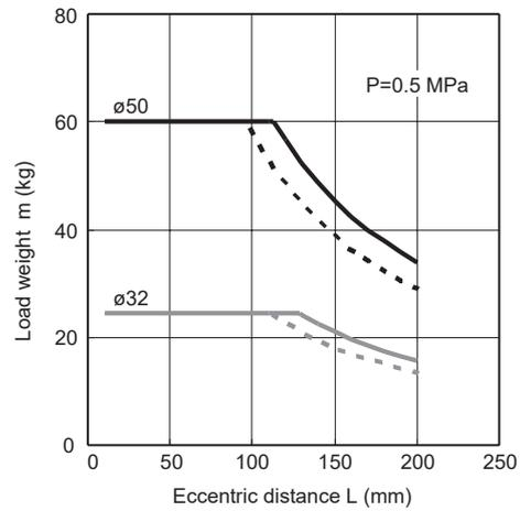
\*1 : For operation at low speed, select the model within the dotted line as a guide.
