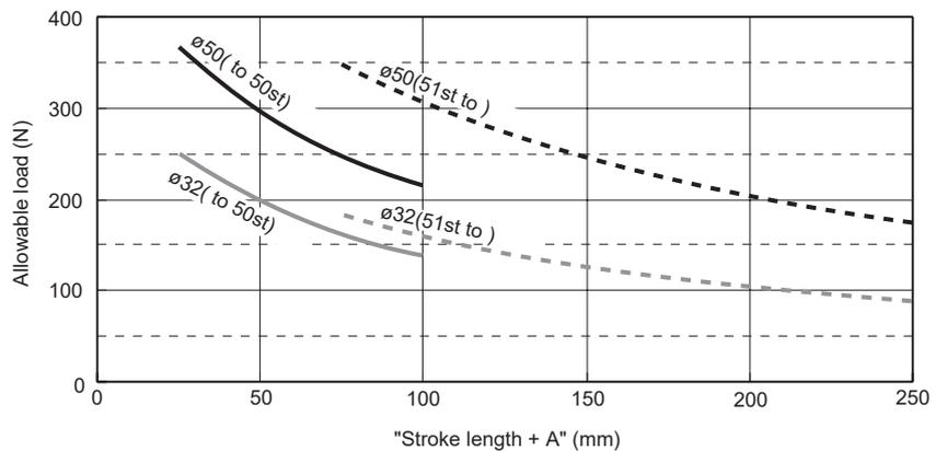
The allowable lateral load is a value for when the load is acting on the end surface of the end plate. When the center of gravity of the workpiece mounted on the end plate will be moved, substitute this distance for the stroke length before selection.
