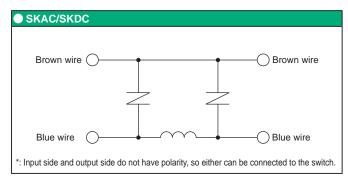
Note: SKAC is for AC circuit only and SKDC is for DC circuit only.
