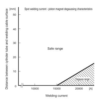
Degaussing occurs when an alternating current magnetic field is applied to the magnet. Measures have been taken for the cylinder with H type switch magnet. While degaussing does not occur up to 15,000 A, at over 15,000 A, provide the above distance between the cylinder tube and welding cable surfaces.
