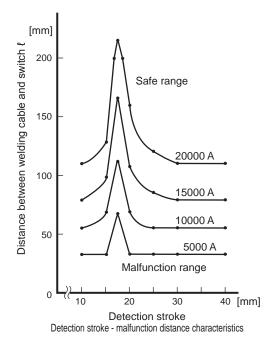
When using with the detection stroke set to 30 mm or less, provide the distance in the figure above between the welding cable and switch.
