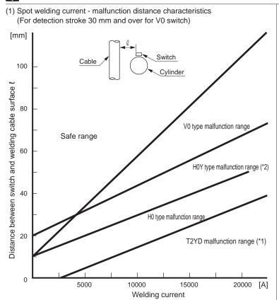
The above external magnetic field resistance properties apply when H0 is installed within the "max. sensitivity position ±1 mm," within the "max. sensitivity position ±1.5 mm" for V0, and within the "optimum installation range" for H0Y. Install switches within this range. Do not apply welding current to flow during movement of the cylinder piston.
