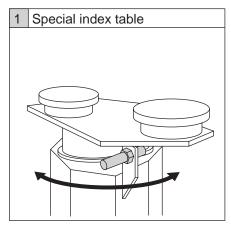
If used for special indexing tables such as wheel rim welding, etc., the index time can be reduced without damaging the machine.
