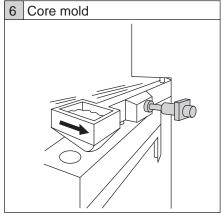
Can be used to stop the swing arm in the process that injects sand model material. This also increases cycles per unit time and supports increases in production.
