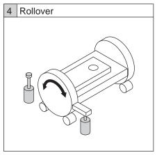
Can be used for automatic turn-over mechanism for parts after machining and welding, etc. Reduces wear and extends the service life of driving parts such as the drive, gears, pinion, etc.
