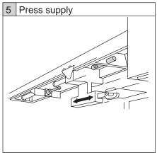
Can be used with feeding mechanisms for parts leading to press machine dies (molds, stamps). Without reducing the supply speed of pneumatic cylinders, etc., the deceleration effects suited for the parts can be attained.
