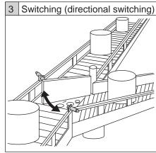
When used for defective parts inspection and sorting for shipping, this mechanism absorbs the gate bound impact and prevents damage to pneumatic cylinders, etc.
