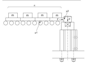
3. Obtain the working pressure from the required thrust (P) using Fig. 3.
