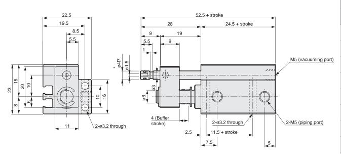
\* Recommended inner diameter tolerance of the mating side's socket: H8
