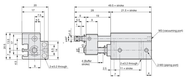
\* Recommended inner diameter tolerance of the mating side's socket: H8
