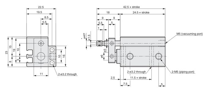
$^{\star}$  Recommended inner diameter tolerance of the mating side's socket: H8  $\,$
