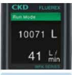
Upper: Accumulated flow Lower: Instantaneous flow rate
