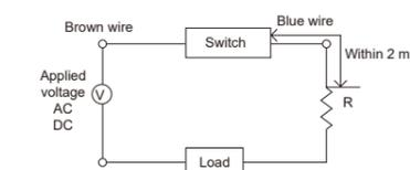
● Inrush current limiting resistor
