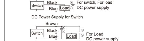
(Connection to Programmable Logic Controller (PLC))
