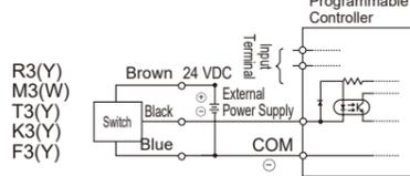
● Example of connection to sink input (external power supply) type
