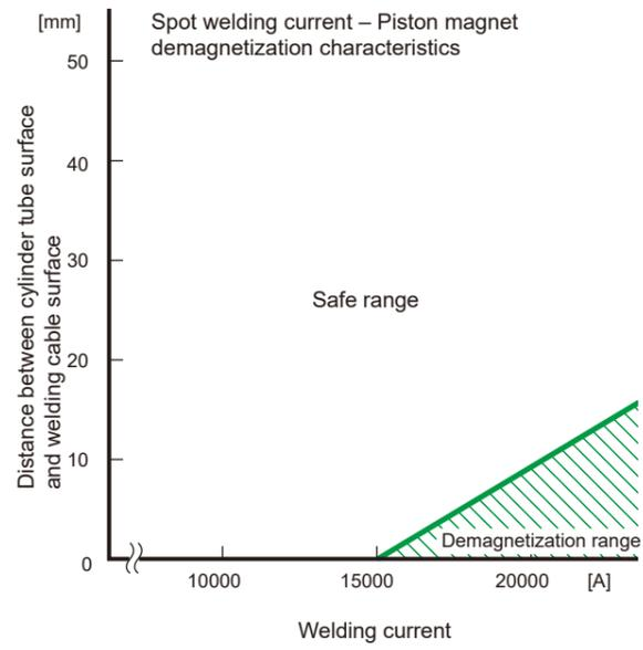
Demagnetization occurs when an AC magnetic field is applied to the magnet. The magnet of the H-type switch equipped cylinder has countermeasures and will not demagnetize up to 15,000 A, but if it exceeds 15,000 A, please maintain the distance shown in the figure above between the cylinder tube surface and the welding cable surface.
