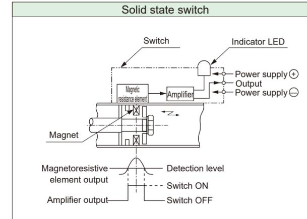
When the piston magnet approaches, a change occurs in the magnetic field, and the output voltage of the magnetoresistive element changes as shown in the figure. By amplifying this signal, a switching output as shown in the figure can be obtained.
