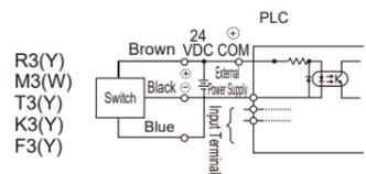
● Connection to source input (built-in power supply) type
