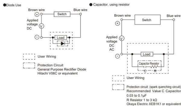
When connecting and using capacitive loads (capacitors), inrush current will occur when the switch is ON, so always install a contact protection circuit.
