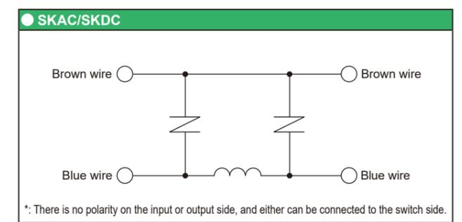
Note: SKAC is exclusively for AC circuits, and SKDC is exclusively for DC circuits.
