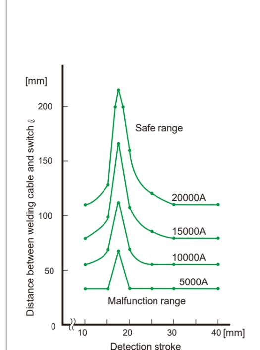
Detection stroke - Malfunction distance characteristics
