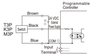
● Example of connection to sink input (built-in power supply) type
