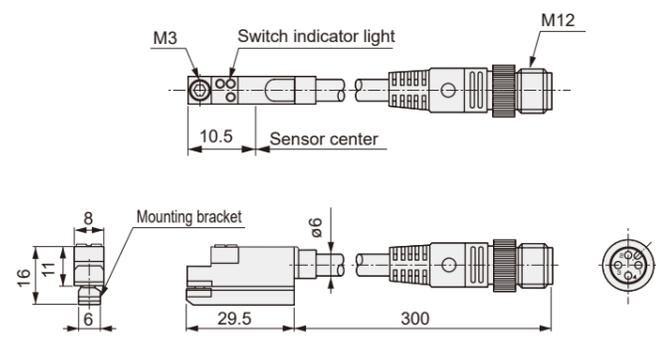
External dimension diagram / Switch internal circuit diagram
