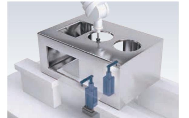
Workpiece auxiliary holding for transfer robots
