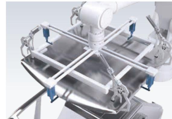
Workpiece clamping with welding jigs
