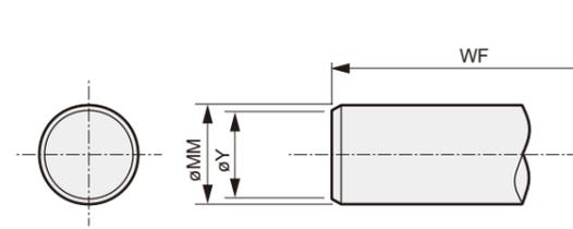
\*1: "WF" is not listed in the SCP\*3 catalog. The "13 mm" dimension should be taken as "WF".
