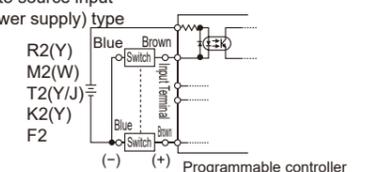
● Connection to source input (built-in power supply) type
