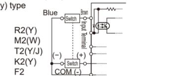
● Connection to sink input type Programmable Controller
