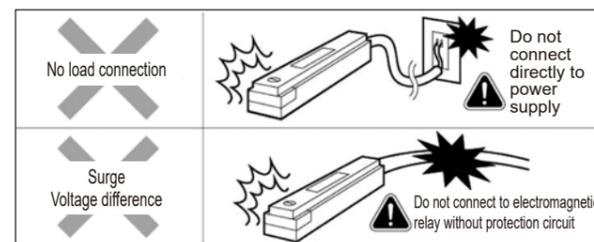
■ For electromagnetic relays and long wiring, install a "protection circuit."
