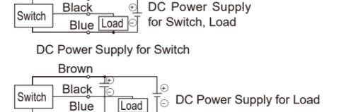
(Connection to Programmable Logic Controller (PLC))
