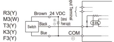
● Example of connection to sink input (external power supply) type
