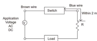
● Inrush current limiting resistor
