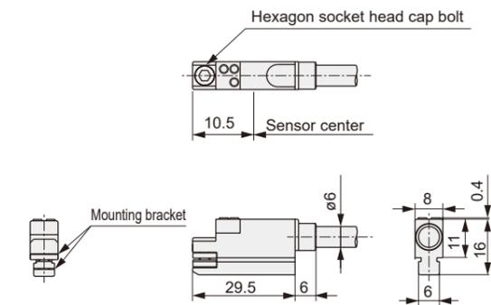
●T2YDU (Switch for AC magnetic field with M12 cable connector)
