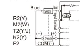
● Connection to sink input type Programmable Controller
