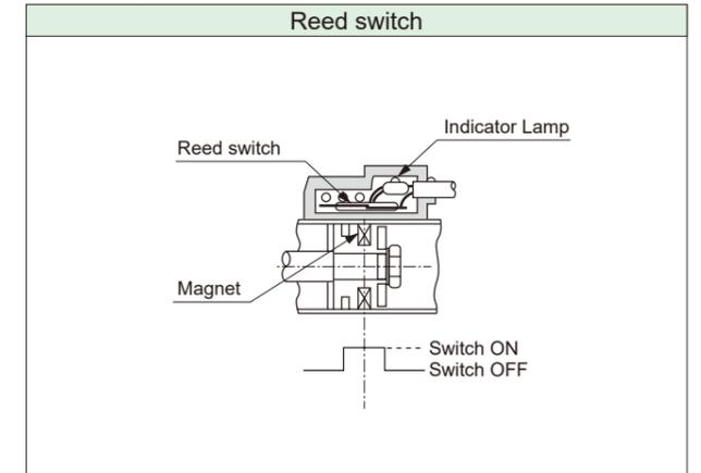
When the piston magnet approaches, a magnetic field is generated, the opposing contacts of the reed switch are magnetized, an attractive force is generated, and the contacts close.
