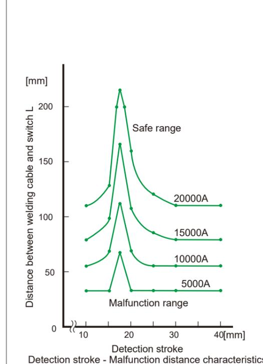
Detection stroke - Malfunction distance characteristics
