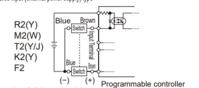
● Connection to source input (built-in power supply) type Programmable controller
