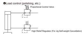
\*To improve supply/exhaust characteristics, maximize piping volume as much as possible.
