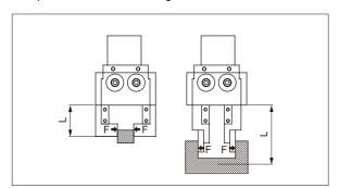
Performance data indicates the gripping force at hand finger length L at a supply pressure of 0.15 to 0.7 MPa.
