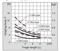
When determining the gripping force from performance data, if L is the distance to the workpiece's center of gravity when the attachments are manufactured, the gripping force F is as follows
