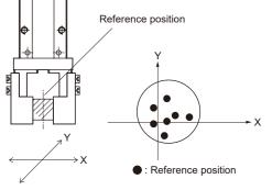
cylinder piston position, and it is conceivable that its value will fluctuate due to deformation/wear of the jig, etc., over the course of use. (In the case of a gripper, backlash in the opening/closing direction of the finger part and deformation/wear of the attachments are contributing factors to variation.) If the analog output voltage fluctuates, make fine adjustments with the zero point adjustment external trimmer as necessary.
