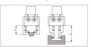
The performance data shows the gripping force at Finger length L of the gripper at a supply pressure of 0.15 to 0.7 MPa.
