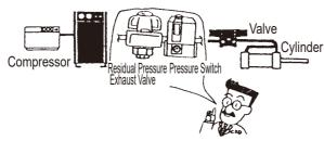
■The load factor for fall prevention cylinders should be 50% or less.
