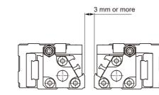
■ When using locating holes, use pins with dimensions that do not result in a press fit. Using press-fit dimension pins may cause damage to the linear guide part due to press-fitting load or accuracy deterioration due to distortion. The recommended tolerance for the pin is JIS tolerance m6 or less.
