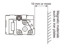
■ If cylinders are adjacent as shown in the diagram below, the cylinder switch may malfunction. Maintain the following distance from the cylinder surface. (Common to all bore sizes)
