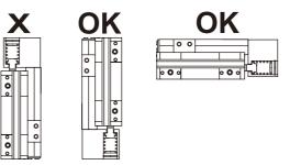
■Use the buffer with a stroke less than the buffer stroke. This will cause malfunction or damage.
