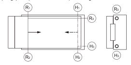
(R) indicates the rod side pressurizing port, and (H) indicates the head side pressurizing port. At the time of factory shipment, ports other than (R) (H) (R2 (H2) depending on the stopper position when a stopper is selected) are sealed with plugs.
