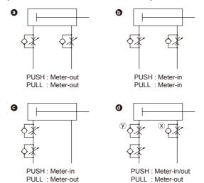
When driving a single-rod cylinder at creep speed in the PUSH direction, if the load resistance is small, a flying-out phenomenon may occur at the start of operation. As a countermeasure, use circuits (b), (c), (d). Note that circuit **d** is the most stable.
