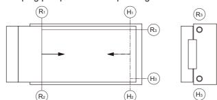
(R) indicates the rod side pressure port, and (H) indicates the head side pressure port. At the time of factory shipment, ports other than (R1) (H1) (depending on stopper selection and stopper position (R2) (H2) are sealed with plugs.
