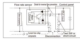
■ Take the following measures to prevent damage caused by reverse current:
