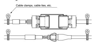
■ Do not fix the cable leading out of the actuator in a pulled state.
