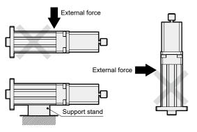
To prevent breakage of the piston rod end thread, wear of the bushing, seizure, etc., connect the piston rod end and the load with a free joint or simple flow controller so that there is no twisting at any position of the stroke.
