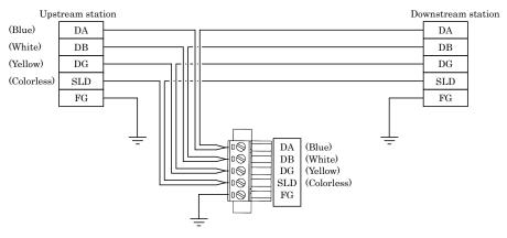
\* The figure above shows multidrop wiring diagram. For T-junction connection diagram, refer to the master station user's manual.
