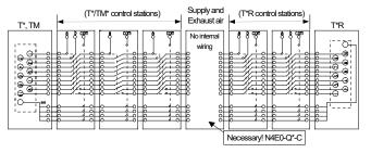
Example of incorrect layout: Left and right wiring interfere at the center
