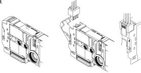
When the power input socket is engaged, valve internal wiring is temporarily disconnected from the reduced wiring on the manifold, enabling external power supply.
