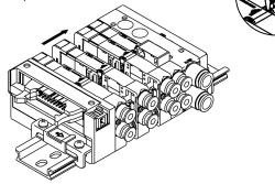
Raise the block on electric cover side and pull it toward the piping port to remove it from DIN rail.
