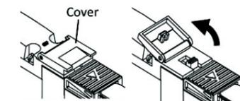
Operating method of The device which release residual pressure.
