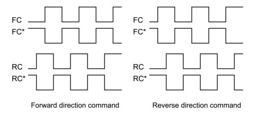
Figure 3-3 90 deg phase difference signals
