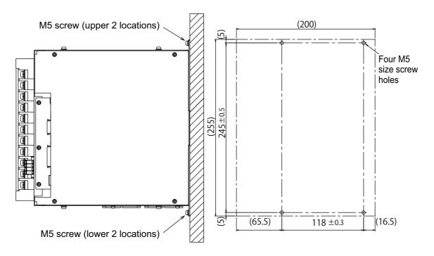
Figure 2-6 Device installation method (7 kW)
