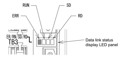
Figure 1-3 Data link status display LED panel
