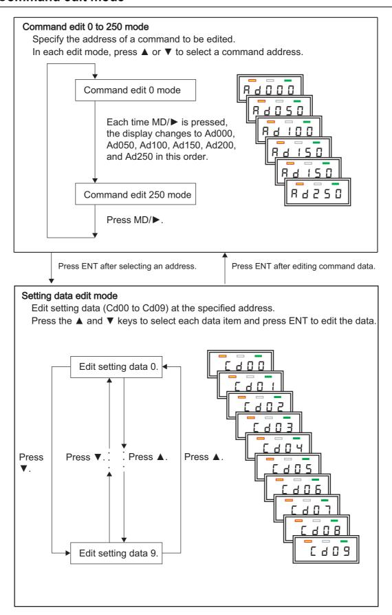
Figure 12-9 Command edit mode configuration and transition
