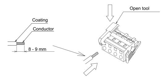
Figure 2-16 Plug connector wiring diagram (400 V and 7 kW)
