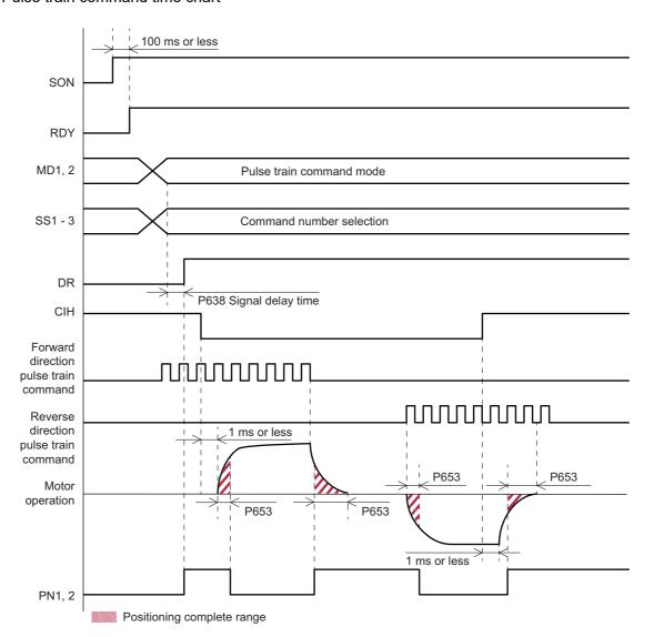
Figure 5-5 Pulse train command time chart
