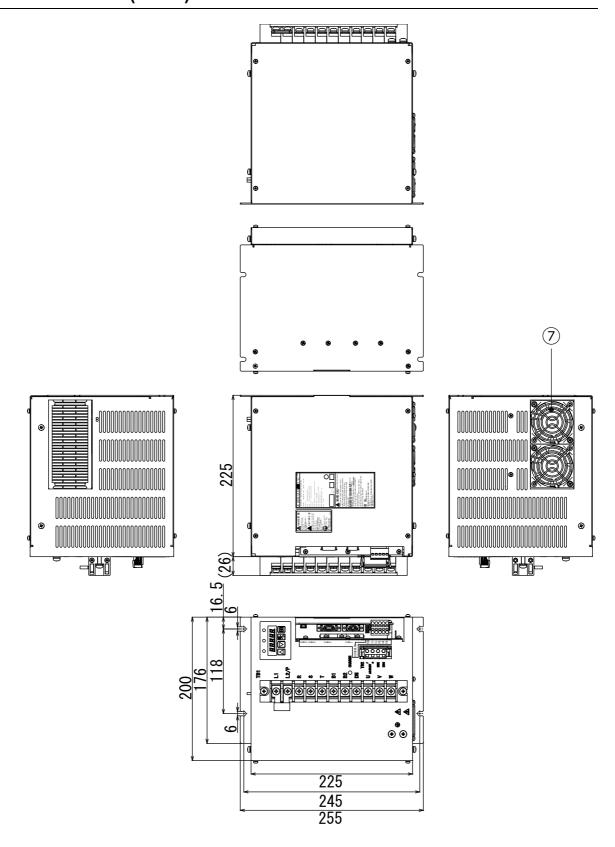
Figure 13-13 Outline drawing of the main unit of the device with 400 V and 7 kW (Type 7)
