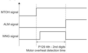
**c.** If the detection specification is "No warning"and the detection time is "1 to 999" After the period during which the MTOH signal is continuously ON reaches the set time,
