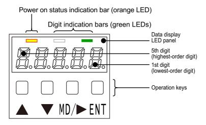
Figure 12-1 Configuration of the operation panel
