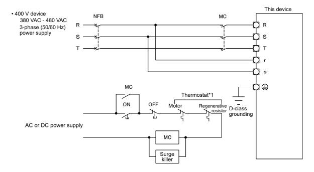
Figure 2-9 Typical power supply circuit for 3-phase power supply (400 V device)
