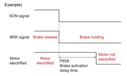
② If the servo on signal (SON) is OFF (if it is held OFF for a time shorter than the [P658 (8th - 5th digits)] setting)
