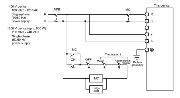
Figure 2-10 Typical power supply circuit for single-phase power supply
