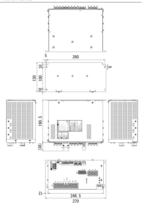
Figure 13-7 Outline drawing of the main unit of the device with 3.3 kW (Type 4)
