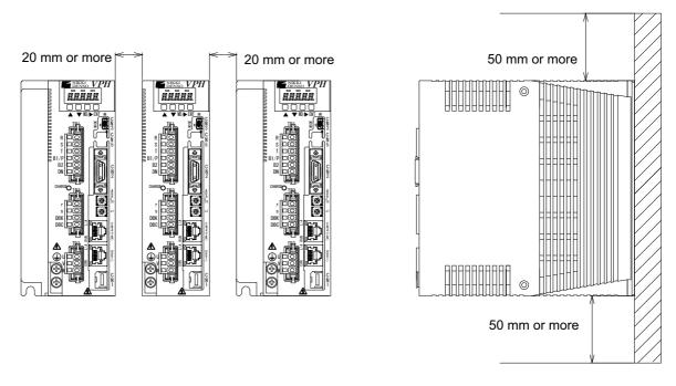
Figure 2-2 Installation and ventilation of the device
