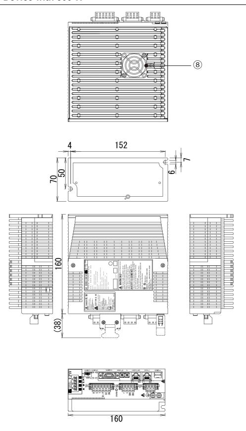
Figure 13-3 Outline drawing of the main unit of the device with 800 W (Type 2)
