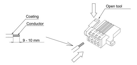
Figure 2-14 Plug connector wiring diagram (800 W or less)
