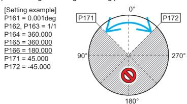
\* If the rotation position range is set, software overtravel may not be detected normally. Thus, in this case, use this function for an auxiliary use of overtravel detection with a sensor (such as a limit switch).
