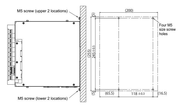
Figure 2-6 Device installation method (7 kW)
