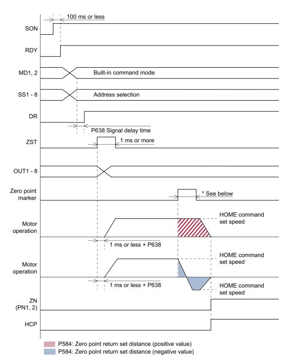
\* Select the zero point marker to use from [P581 (1st digit): Zero point marker selection for homing].
