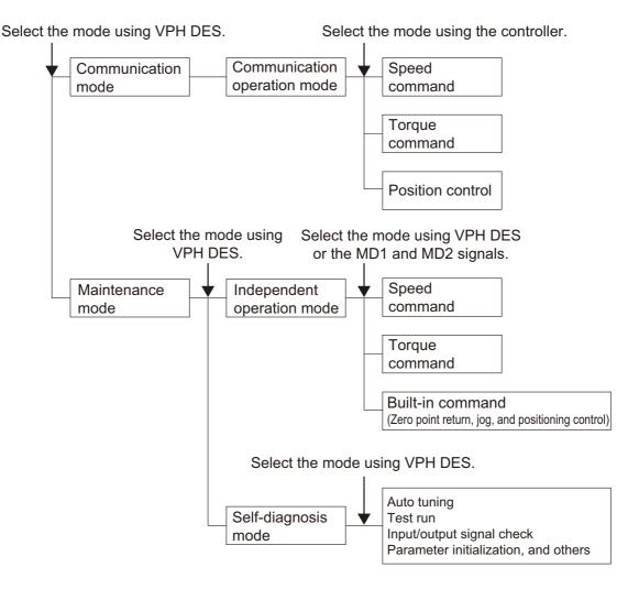
Figure 1-5 Mode configuration diagram
