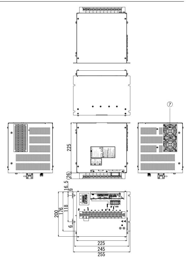
Figure 13-13 Outline drawing of the main unit of the device with 400 V and 7 kW (Type 7)
