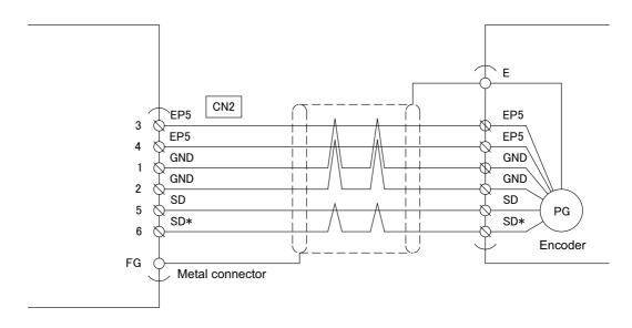
Figure 3-2 Serial encoder connecting diagram
