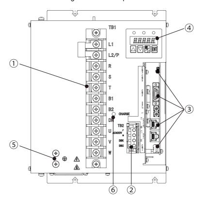
Figure 13-14 Front view of the main unit of the device with 400 V and 7 kW (Type 7)
