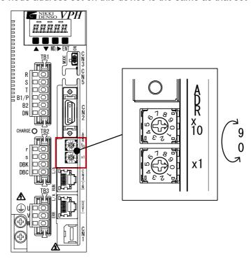
Figure 1-3 Node address selection switch
