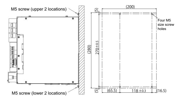
Figure 2-7 Device installation method (15 kW)
