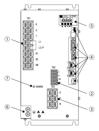
Figure 13-8 Front view of the main unit of the device with 3.3 kW (Type 4)
