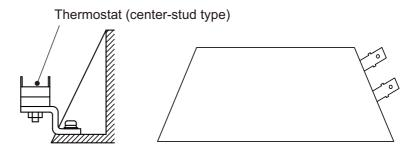
Figure 2-12 Mounting a thermostat on a cement resistor
