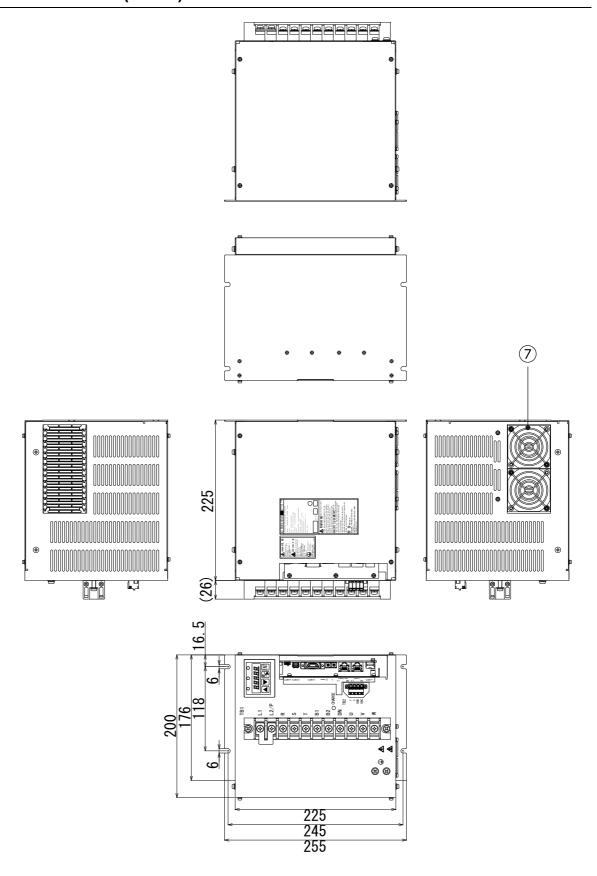
Figure 13-9 Outline drawing of the main unit of the device with 200 V and 7 kW (Type 5)
