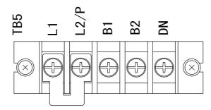
When not using a DC reactor, do not remove the shorting bar between L1 and L2/P. Connect the grounding to the grounding terminal on the device cabinet.
