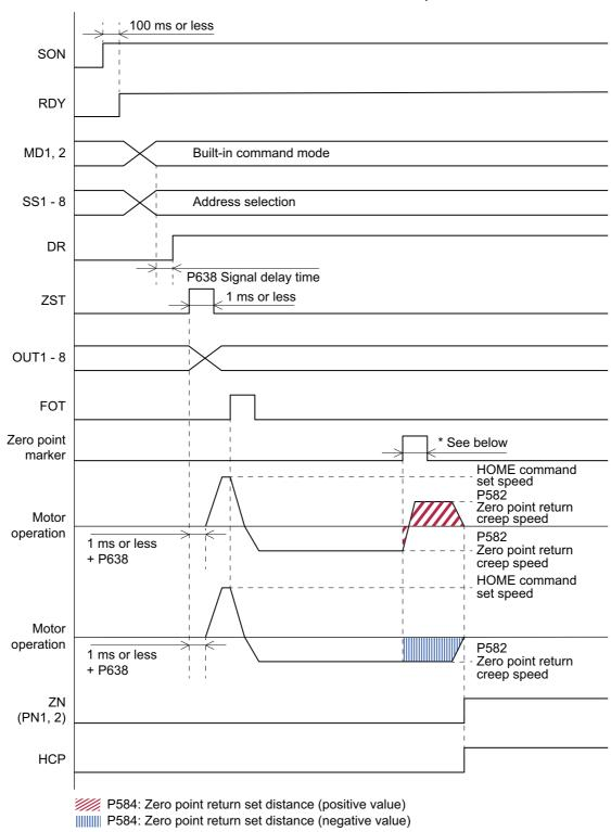
\* Select the zero point marker to use from [P581 (1st digit): Zero point marker selection for homing].
