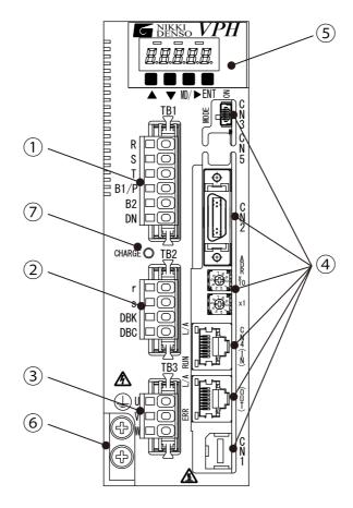
Figure 13-2 Front view of the main unit of the device with up to 400 W (Type 1)
