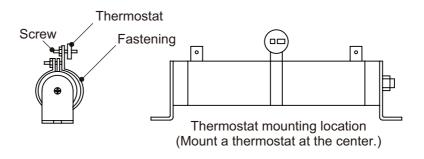
Figure 2-13 Mounting a thermostat on a vitreous enamel resistor
