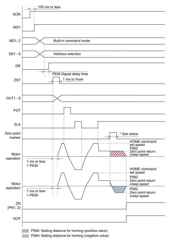
\* Select the zero point marker to use from [P581 (1st digit): Zero point marker selection for homing].
