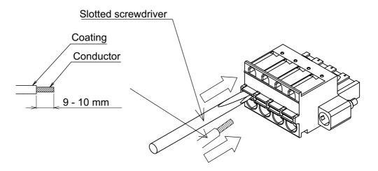
Figure 2-15 Plug connector wiring diagram (200 V and 7 kW, 15 kW)
