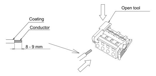
Figure 2-16 Plug connector wiring diagram (400 V and 7 kW)
