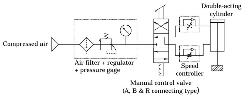
**Fig.3. An example of ABR ports valve circuit combined with a master valve**
