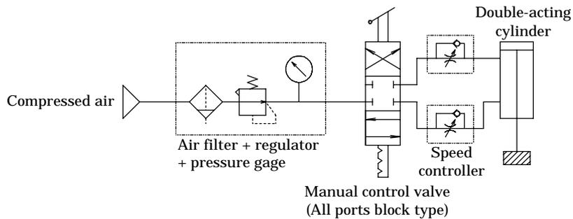
**Fig.2. An example of ABR ports valve circuit**
