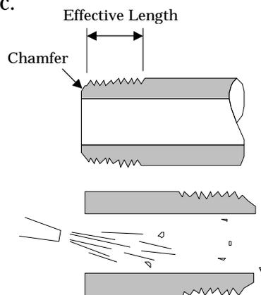
3) Flush air into the pipe to blow out foreign substances and chips before piping.
