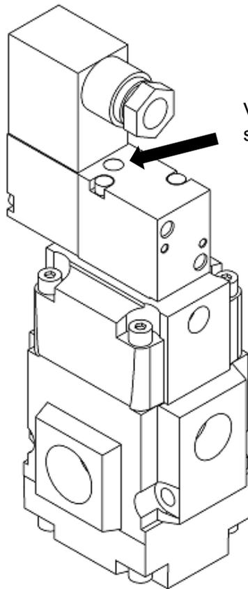
Valve operates while the manual shaft is pushed and held down.
