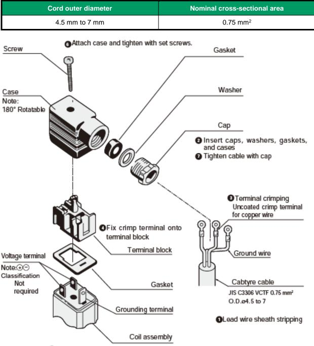
GInsert gasket and terminal block into coil terminal.
