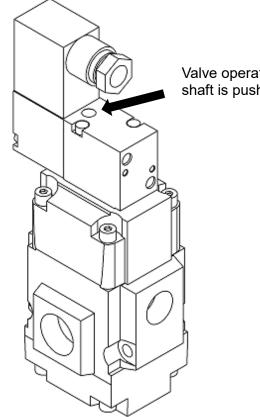
Valve operates while the manual shaft is pushed and held down.
