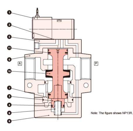
Part No. Part name Material Part No. Part name Material 1 Pilot solenoid valve i-7 Valve seat C3604 Brass NBR 2 Gasket Nitrile Rubber 8 SUS304 Stainless steel Spring POM 3 Piston Acetal resin 9 Cap AC4C Aluminum casting 4 MY packing NBR Nitrile Rubber 10 Valve stem NBR, A2017 Nitrile Rubber, Aluminum 5 Stuffing AC4C Aluminum casting 11 Packing NBR Nitrile Rubber 6 AC4C Aluminum casting Body
