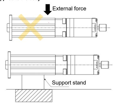
• External force may cause malfunction or damage to parts. Provide a support stand for horizontal front installation. Avoid fixing only with the flange mounting hole.
