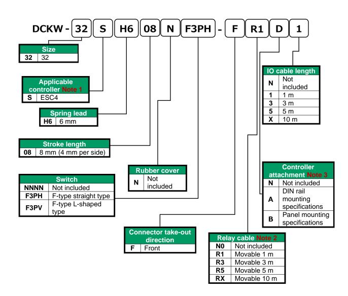
Note 2: Refer to "1.4.4Relay cable, cylinder switch cable", for the external dimensions of the switch cables and relay cables.
