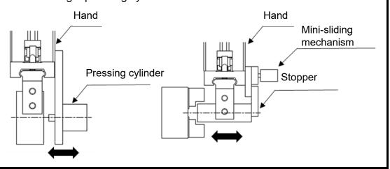
Repeatability refers to the displacement of the finger stop position when clamping and unclamping are repeated under the same conditions. The same conditions include hand fixing and use of the same attachment, as described below.
