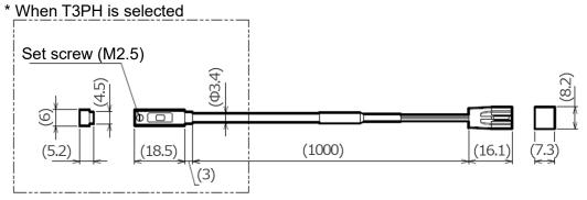
Depending on the switch model number selection, the dotted line part will be as shown below.
