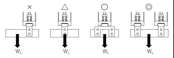
When inserting a workpiece directly into a jig with the hand, consider escape when designing.
