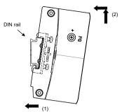
When the screws are loose, move up the operation button and put it on the DIN rail from underneath.
